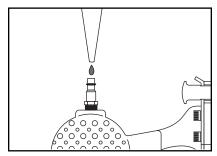
Figure 4. Lubricating nailer via air inlet.
